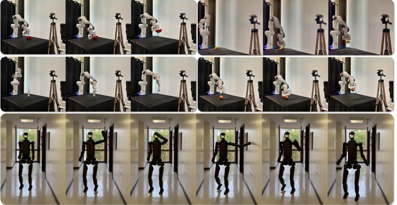
Fig. 12: **Sim-to-Real and Sim-to-Sim-to-Real Experiment Results.** We demonstrate that learning within the RoboVerse framework enables seamless direct Sim-to-Real transfer for manipulating unseen objects in new environments (imitation learning) and Sim-to-Sim-to-Real transfer for whole-body humanoid control (reinforcement learning).
