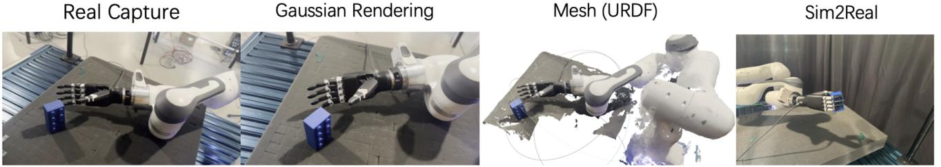
Fig. 20: Visualization of our real2sim pipeline for robotic grasping.
