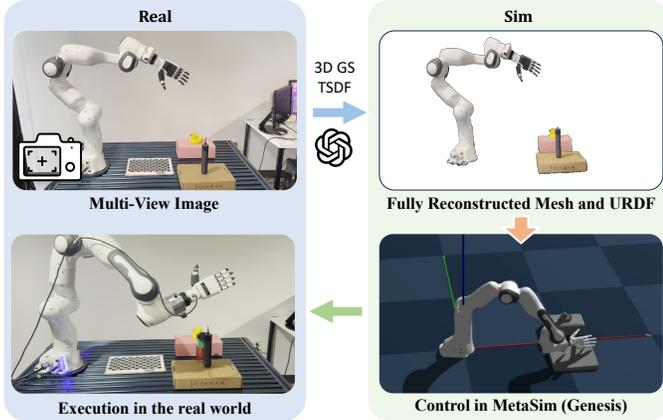
Fig. 7: **Real-to-Sim Tools.** We use a mobile device to capture multi-view images, reconstruct a high-quality mesh, build a URDF using VLM, and then perform actions in both RoboVerse and the real world.
