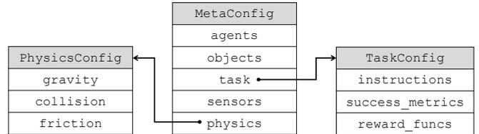
Fig. 4: The MetaConfig is a nested dataclass that abstracts the core components in any simulation environment in a simulator-agnostic way.
