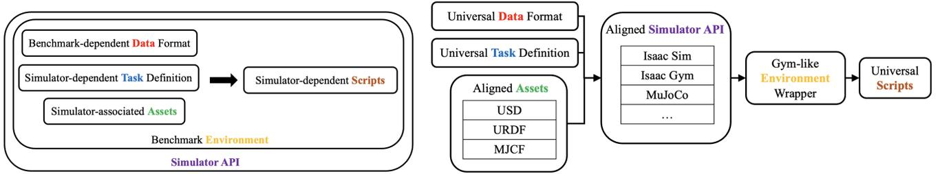
Fig. 15: Comparison between the METASIM and the other simulation environments. Left: Other simulator and benchmark, using self-defined data format, simulator-associated assets, simulator-dependent task definition, and scripts. Right: The METASIM, decoupling all components to be agnostic to specific simulators or benchmark environments.
