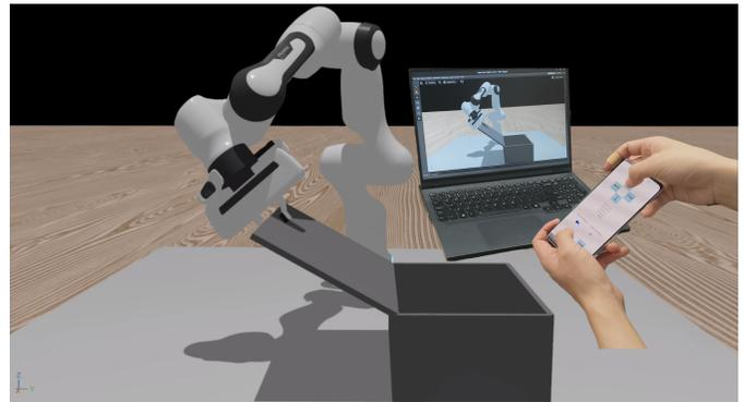
Fig. 19: The smartphone app enables 6-DoF control using orientation sensing and multi-touch buttons for translation commands, while the simulated robot’s movements are visualized in real-time on the workstation.
