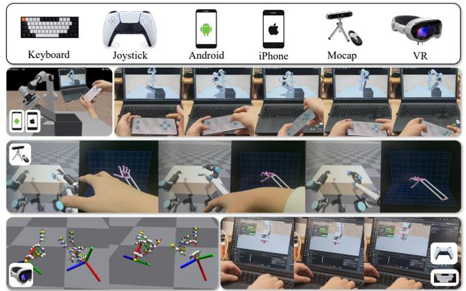
Fig. 5: **Teleoperation System**. ROBOVERSE supports various user-friendly teleoperation approaches. Currently, it enables teleoperation via a phone app (second row), motion capture (middle), VR devices (bottom left), as well as keyboard and joystick (bottom right). These methods allow control of robotic arms, dexterous hands, and bimanual systems across different simulators.
