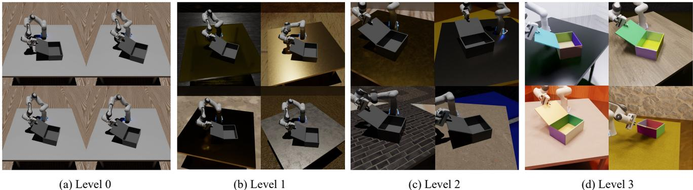
Fig. 9: **Benchmark Protocol:** We define a four-level generalization benchmarking protocol, allocating 90% of the data for training and 10% for generalization evaluation. From left to right, Levels 0 to 3 corresponds to task space generalization, environment randomization, camera randomization, lighting and reflection randomization, respectively.
